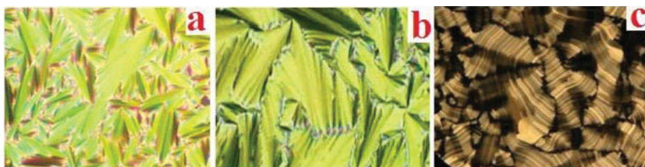
Figure 1. Microphotographs obtained in between the crossed polars. (a) Focal conic fan-shaped texture of smectic-A (Lamellar) phase (250 \times ). (b) Paramorphic fan-shaped texture of highly ordered smectic-B phase (250 \times ). (c) Focal conic fans with radial striation of smectic-E phase (250 \times ).
